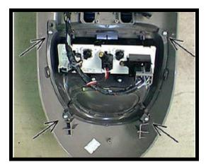
1. Remove and retain OEM front control head bezel assembly by removing four ( 4 ) screws. See Fig. 8.
